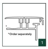
1. For installation of the Incizo profile on stairs or steps, an aluminium subprofile is needed. This subprofile is to be ordered separately (NEVINCPBASE(-)). Do not use the plastic rail included in the Incizo packaging.
